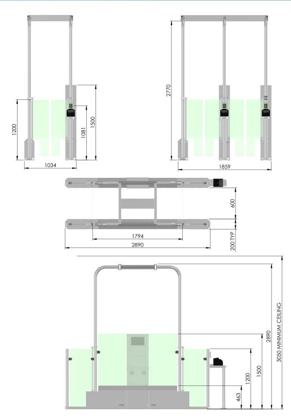
Concrete Base to specification at least (cube) 300N/mm $^2$  of resistance. Base to be flat and level to +/- 5mm over footprint area.
